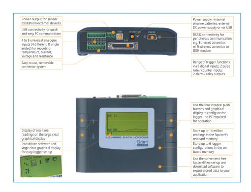
The Squirrel 2010 is a versatile, general purpose data logger, with 4 to 8 analogue input channels to measure current, voltage, resistance and temperature; plus 8 digital channels to automatically trigger or stop logging. An RS232 port is included, allowing connection to modems and other networking devices.
